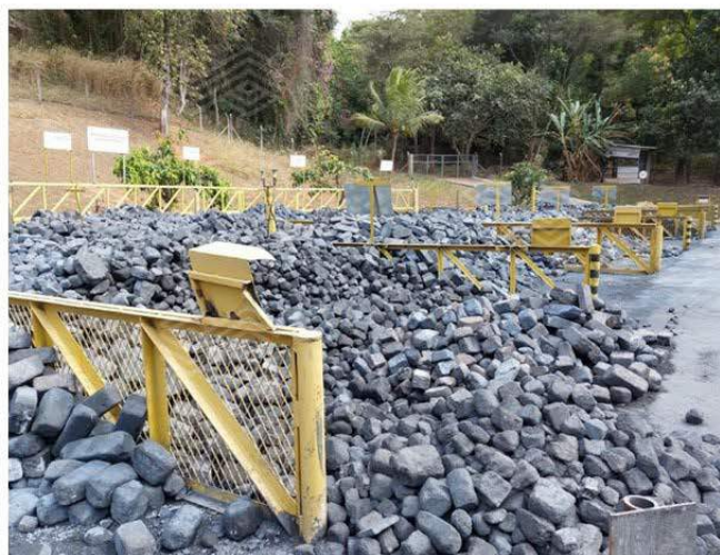
Figure 3. Carbide stabilisation using the weathering method.
